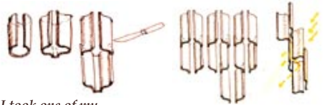
I took one of my favourite devices - the mirrored light-pipe - slit it & slid it down.
