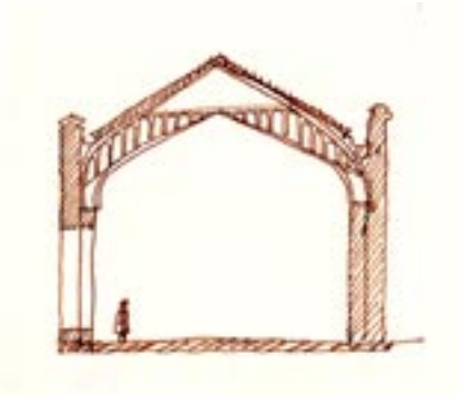
Section through the Hall of Edward III showing the 'naked roofing' of Secular Gothic.
