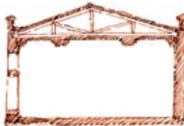
Comparison between the Mediaeval Gothic roof of exposed construction and the hidden structure of the Neo-Classical and Neo-Gothic ceilings.
